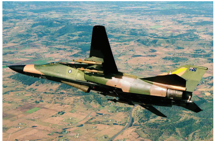
An F-111 fitted with Pave Tack and laser guided bombs, near Amberley Photo: RAAF
